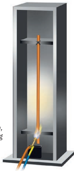
Test of vertical flame propagation, self-extinguishing
