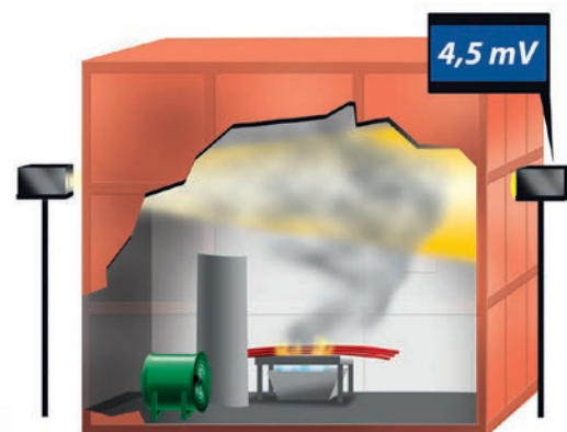
Measurement of smoke density
