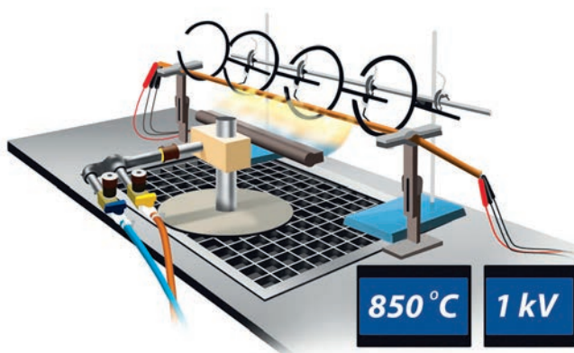
Testing according to EN 60331 (850°C 1 kV)
